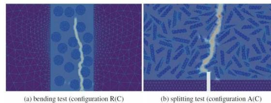
Fracture analysis of aggregate influence on mechanical properties of mortar samples.
