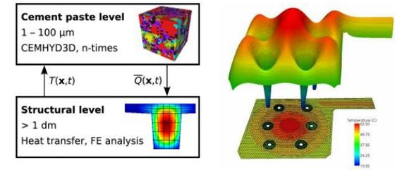
Hydrating concrete produces a significant amount of hydration heat, causing several problems in massive elements. The multiscale simulation helped to find an optimal position of cooling pipes and cooling regime on an arch of Opárno bridge, Czech Republic.
