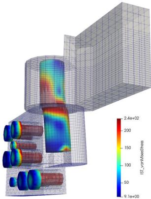
Illustration of nonlinear analysis of a hinge holding hermetic door in an atomic power plant. The model with J2 plasticity without hardening helped evaluating the amount of dissipated energy in the case of a vapour explosion.
