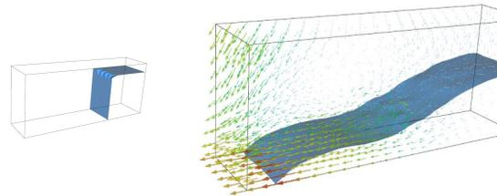
Broken dam problem solved as a problem of two immiscible fluids (water and air) with 3D VOF interface tracking.
