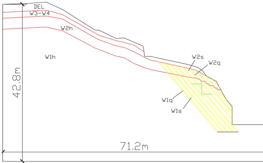
Figure 4.5: Geological situation with plotted footing base in pier No. 10. surroundings. The description of every stratum with material parameters is given in Tab. (4.1)
