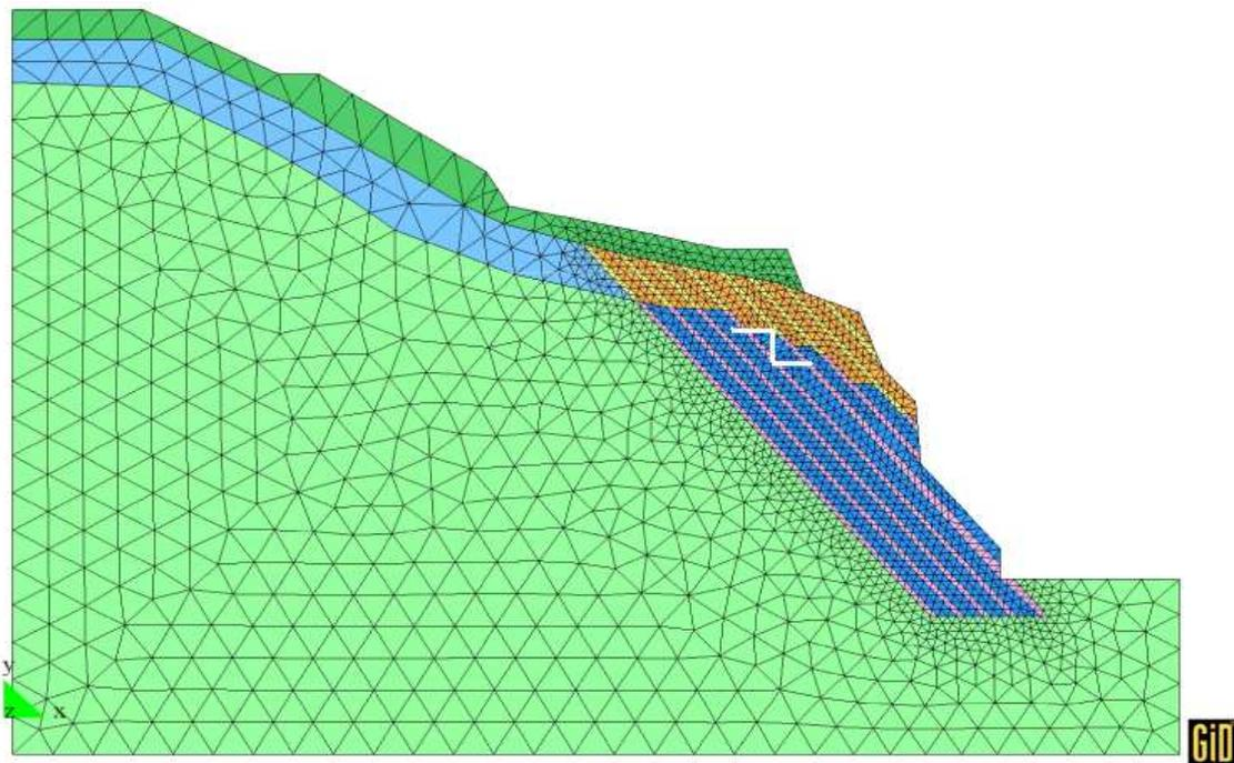
Figure 4.13: 2D mesh of finite elements for the segments of piers 12 with plotted footing base
