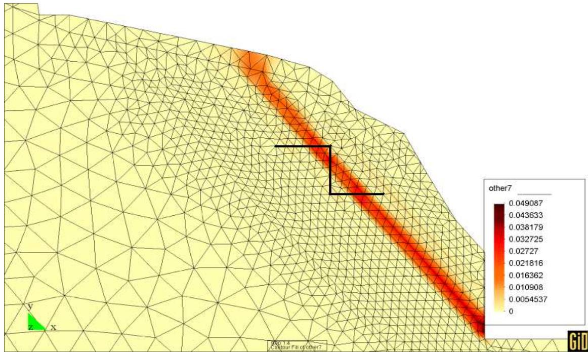
Figure 4.17: Segment of pier No. 10 (load combination 2, reached load factor  $\lambda_f = 1.4$ ) : Detail of plastic zones - values of consistency parameter
