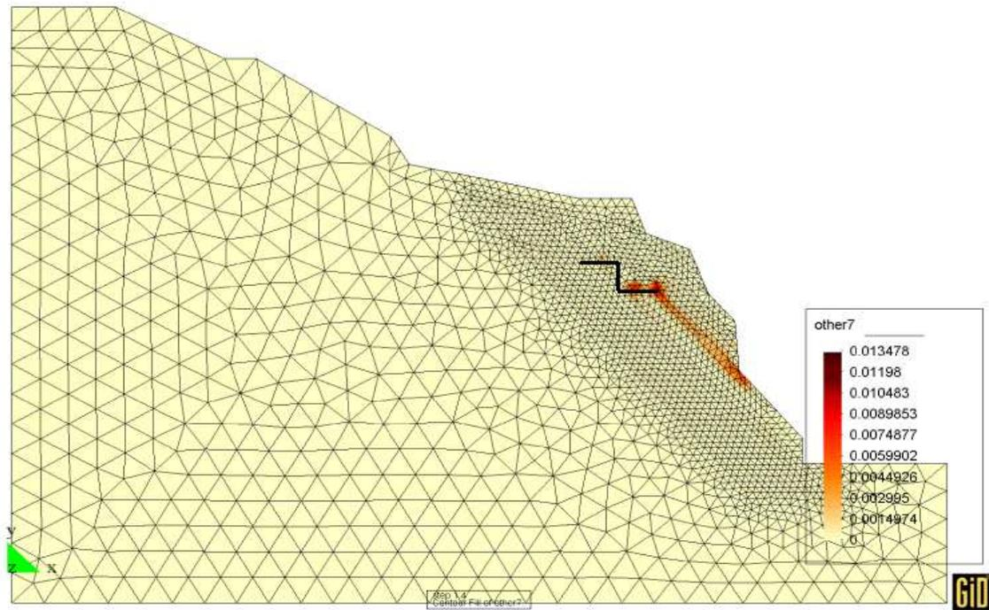
Figure 4.28: Segment of pier No. 12 (load combination 2, reached load factor  $\lambda_f = 1.4$ ) : Plastic zones - values of consistency parameter
