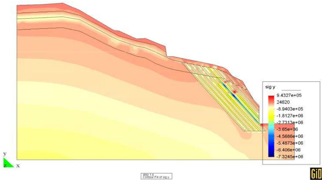
Figure 4.20: Segment of pier No. 10 (load combination 2, reached load factor  $\lambda_f = 1.4$ ) : Vertical stresses  $\sigma_x$
