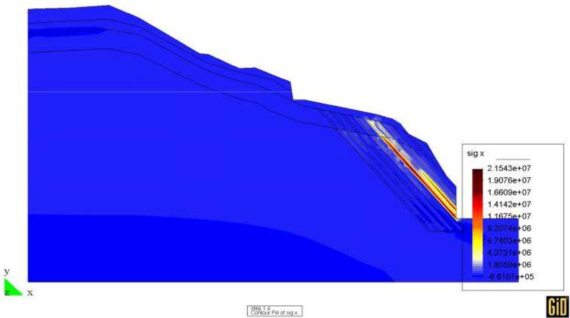
Figure 4.19: Segment of pier No. 10 (load combination 2, reached load factor  $\lambda_f = 1.4$ ) : Horizontal stresses  $\sigma_x$
