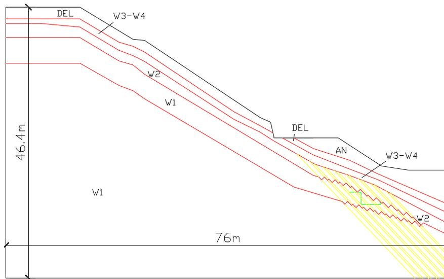
Figure 4.4: Geological situation with plotted footing base in pier No. 4. surroundings. The description of every stratum with material parameters is given in Tab. (4.1)
