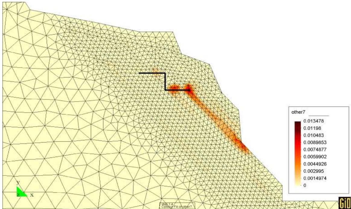
Figure 4.29: Segment of pier No. 12 (load combination 2, reached load factor  $\lambda_f = 1.4$ ) : Detail of plastic zones - values of consistency parameter
