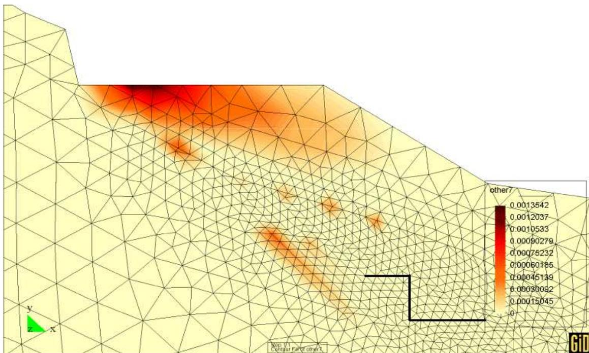
Figure 4.23: Segment of pier No. 4 (load combination 1, reached load factor  $\lambda_f = 1.1$ ) : Detail of plastic zones - values of consistency parameter
