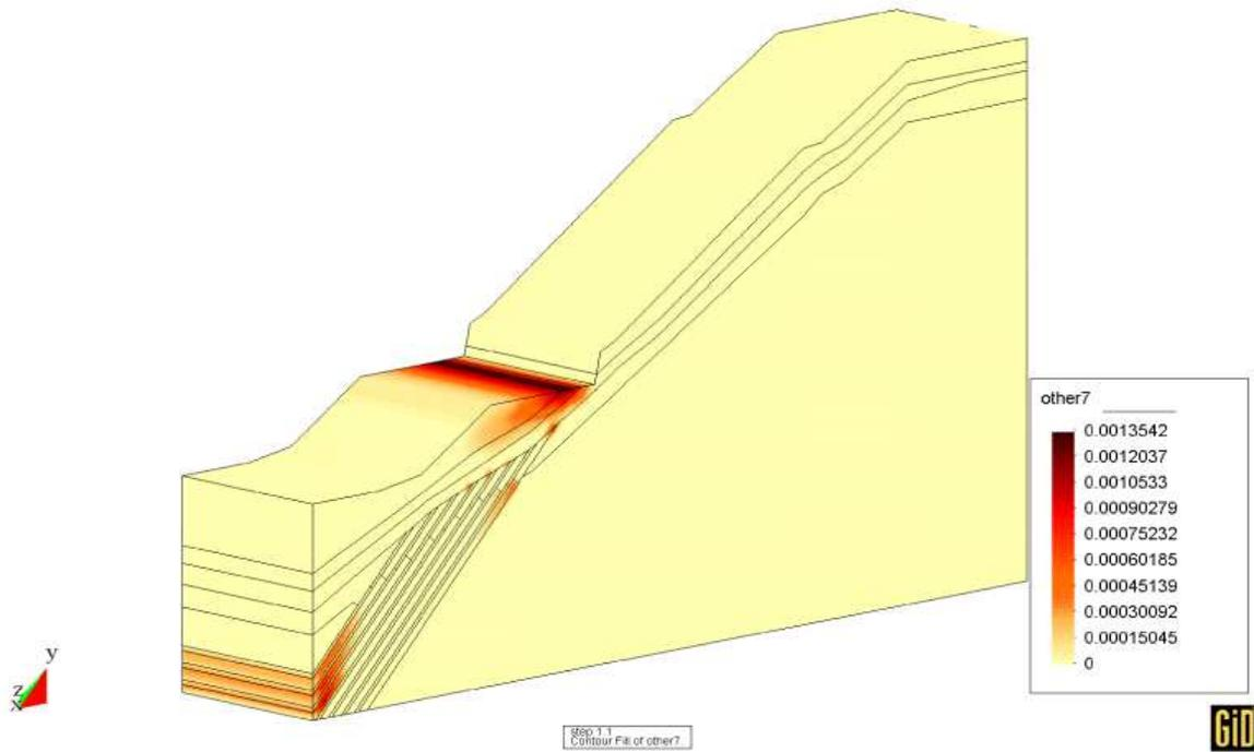
Figure 4.22: Segment of pier No. 4 (load combination 1, reached load factor  $\lambda_f = 1.1$ ) : Plastic zones - values of consistency parameter
