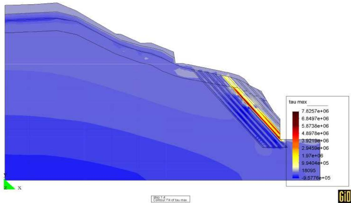
Figure 4.21: Segment of pier No. 10 (load combination 2, reached load factor  $\lambda_f = 1.4$ ) : Principal shear stresses  $\tau_{max}$
