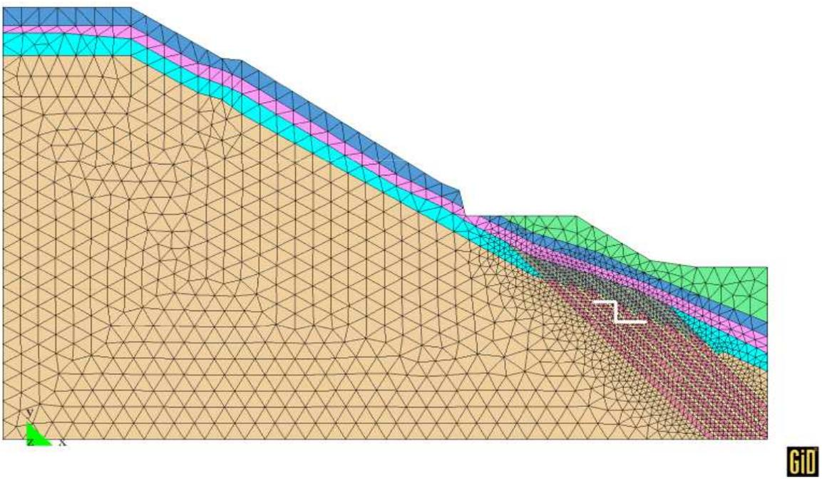
Figure 4.9: 2D mesh of finite elements for the segment of pier No. 4 with plotted footing base
