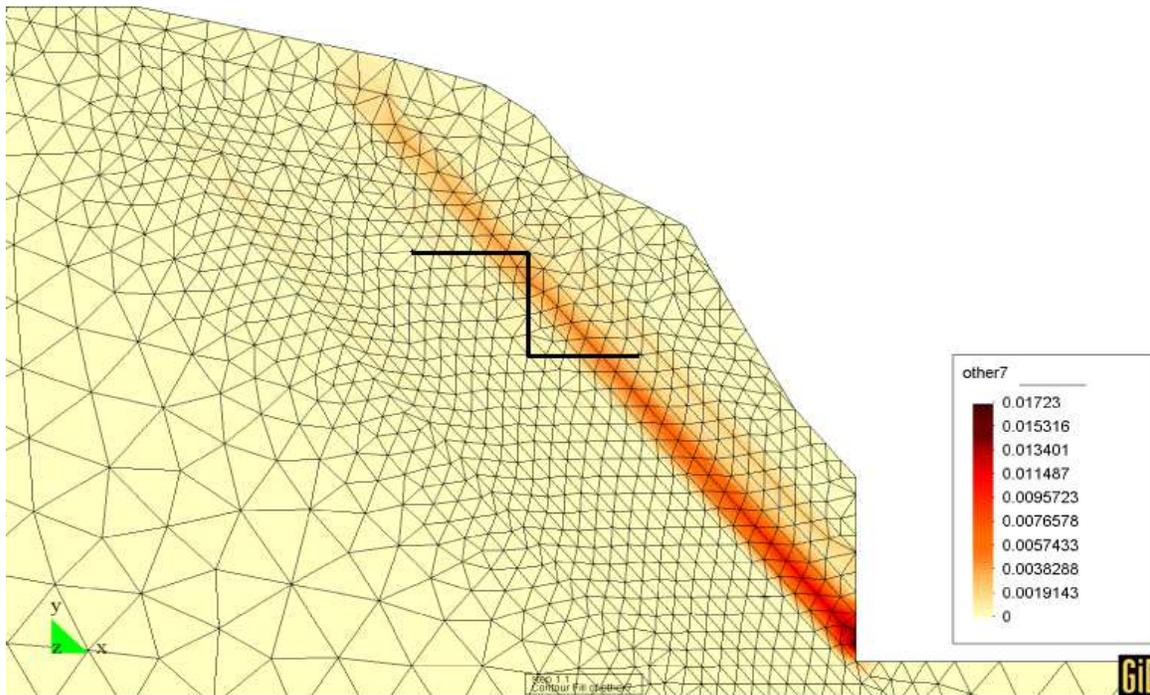
Figure 4.15: Segment of pier No. 10 (load combination 1, reached load factor  $\lambda_f = 1.1$ ) : Detail of plastic zones - values of consistency parameter
