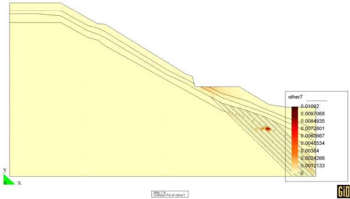
Figure 4.24: Segment of pier No. 4 (load combination 2, reached load factor  $\lambda_f = 1.4$ ) : Plastic zones - values of consistency parameter
