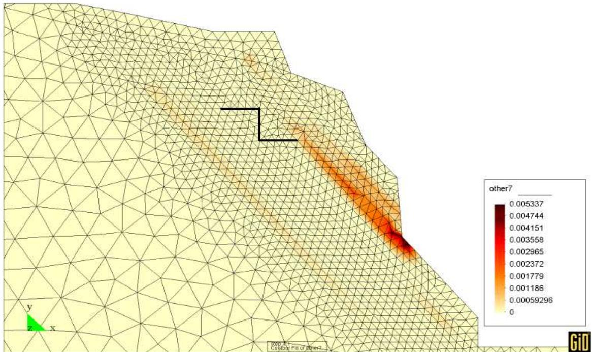
Figure 4.27: Segment of pier No. 12 (load combination 1, reached load factor  $\lambda_f = 1.1$ ) : Detail of plastic zones - values of consistency parameter
