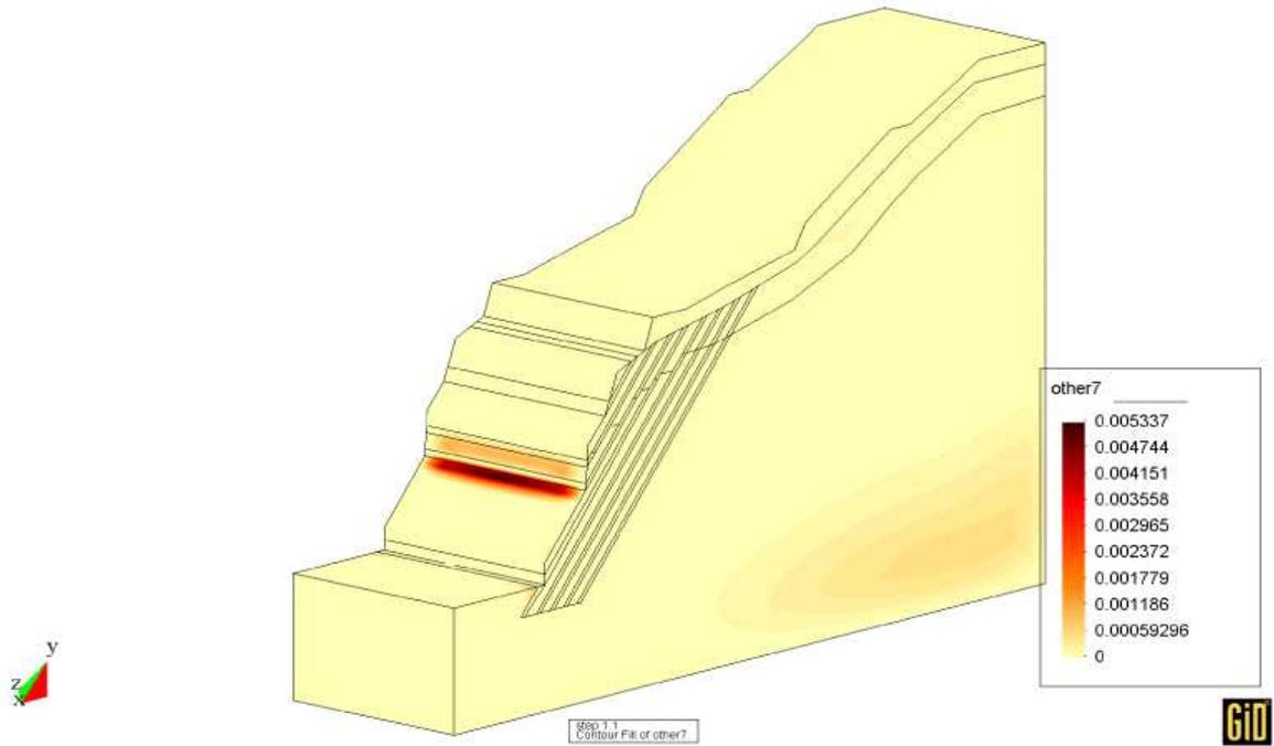
Figure 4.26: Segment of pier No. 12 (load combination 1, reached load factor  $\lambda_f = 1.1$ ) : Plastic zones - values of consistency parameter
