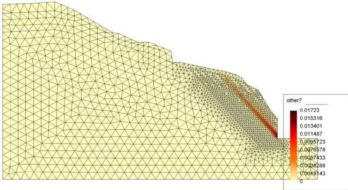
Figure 4.14: Segment of pier No. 10 (load combination 1, reached load factor  $\lambda_f = 1.1$ ) : Plastic zones - values of consistency parameter
