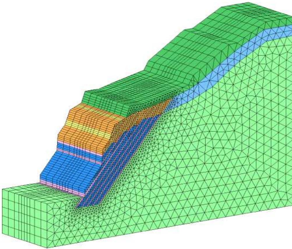
Figure 4.12: 3D mesh of finite elements for the segments of piers 12
