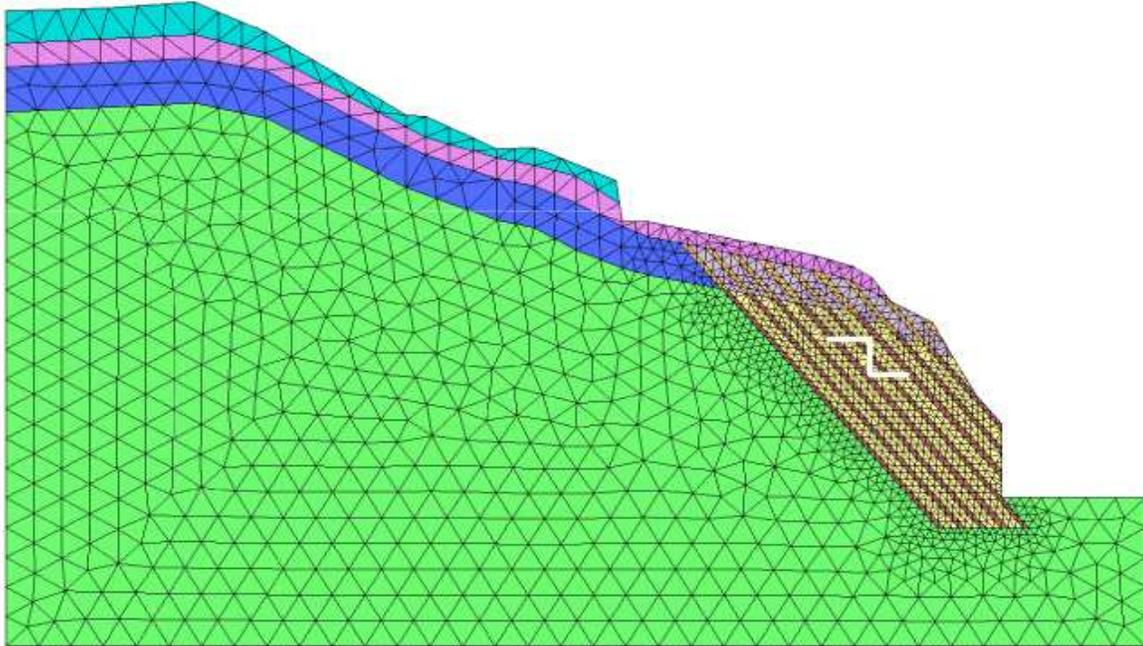
Figure 4.11: 2D mesh of finite elements for the segment of pier No. 10 with plotted footing base
