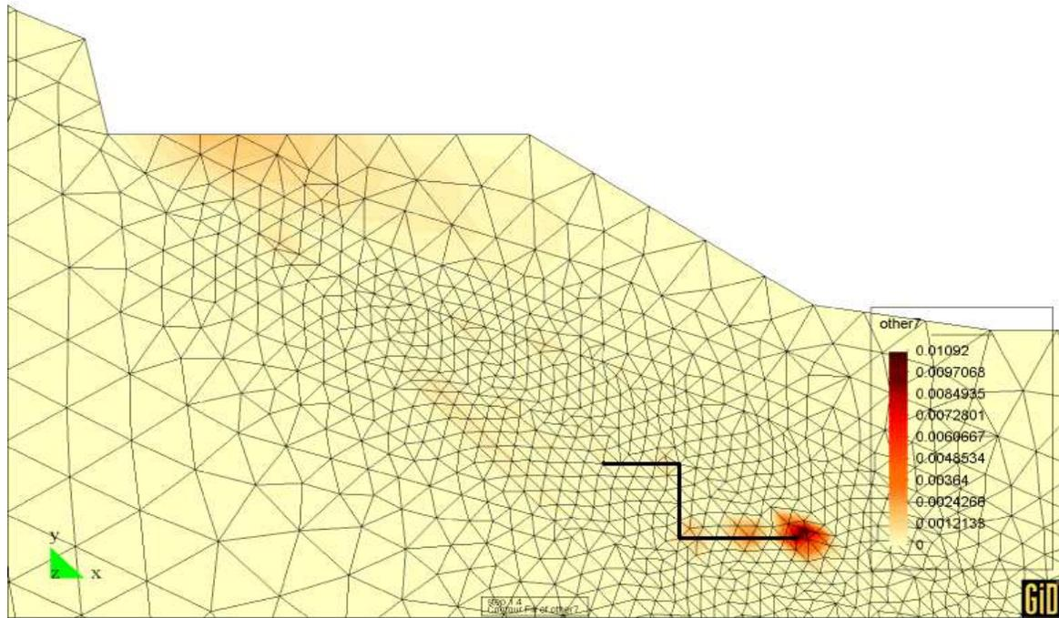
Figure 4.25: Segment of pier No. 4 (load combination 2, reached load factor  $\lambda_f = 1.4$ ) : Detail of plastic zones - values of consistency parameter
