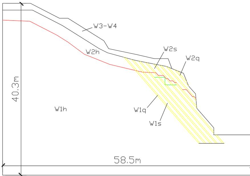
Figure 4.6: Geological situation with plotted footing base in pier No. 12. surroundings. The description of every stratum with material parameters is given by Tab. (4.1)
