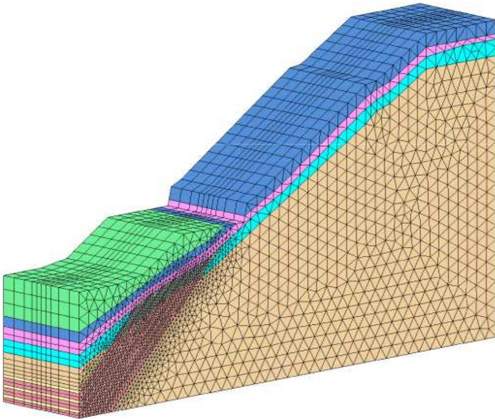
Figure 4.8: 3D mesh of finite elements for the segment of pier No. 4
